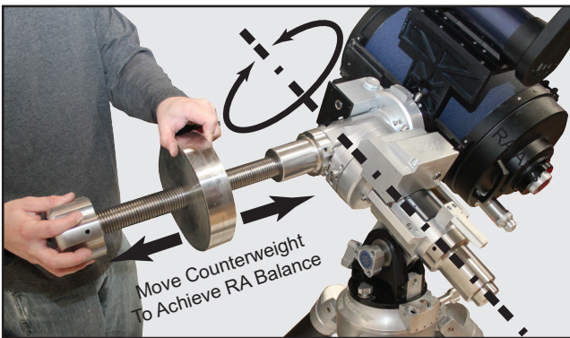
Fig 26: Balancing the RA axes
