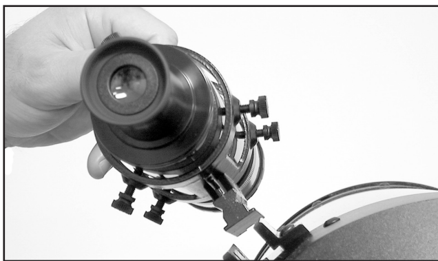
Fig 25: Slide viewfinder into receiver
