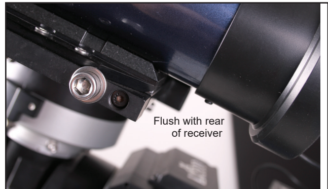
Fig 44: Position StarLock flush with the receiver.
