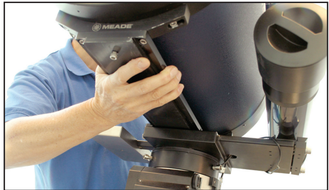
Fig 22: Slide the OTA dovetail into the saddle plate
