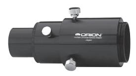
A T-ring (sold separately) is used to match the universal adapter to your particular brand and type of 35mm camera. The adapter attaches to the telescope focuser or eyepiece holder where the eyepiece or diagonal prism would normally be placed. The adapter includes two separate pieces which may be threaded together, the Prime Focus Adapter and the Eyepiece Projection Body.
