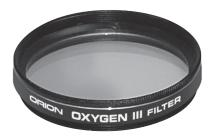
the two doubly-ionized oxygen lines (at 496nm and 501nm) produced by certain types of nebulae. When the OIII filter is threaded onto an eyepiece and used to visually observe one of these nebulae, the image contrast will be greatly increased. You'll be able to observe details you would not normally see!
