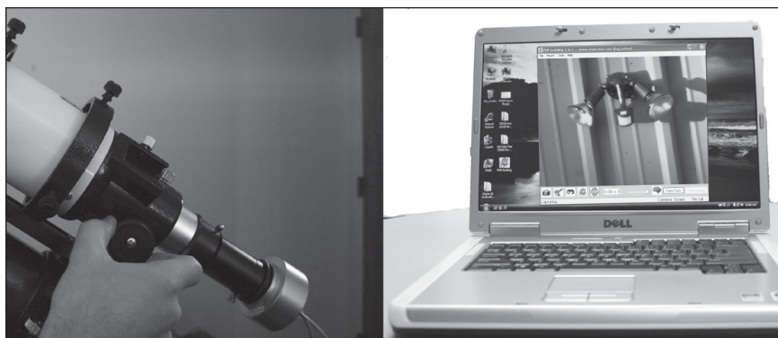
Figure 8. Gradually move the focuser inward until you have a clear daytime image on your computer screen.
