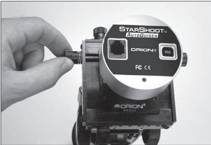
Figure 4.1 and 4.2. Simply turn the position adjustment knobs clockwise or counter-clockwise to move the Guide Star Finder as needed to locate a guide star. (Shown with optional StarShoot AutoGuider, available from Orion.)
