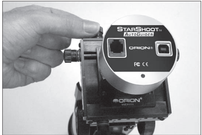
Figure 4.1 and 4.2. Simply turn the position adjustment knobs clockwise or counter-clockwise to move the Guide Star Finder as needed to locate a guide star. (Shown with optional StarShoot AutoGuider, available from Orion.)
