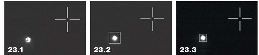
Figure 23.1-23.3. Setting the correct star envelope size is important to ensure the most accurate guiding.
