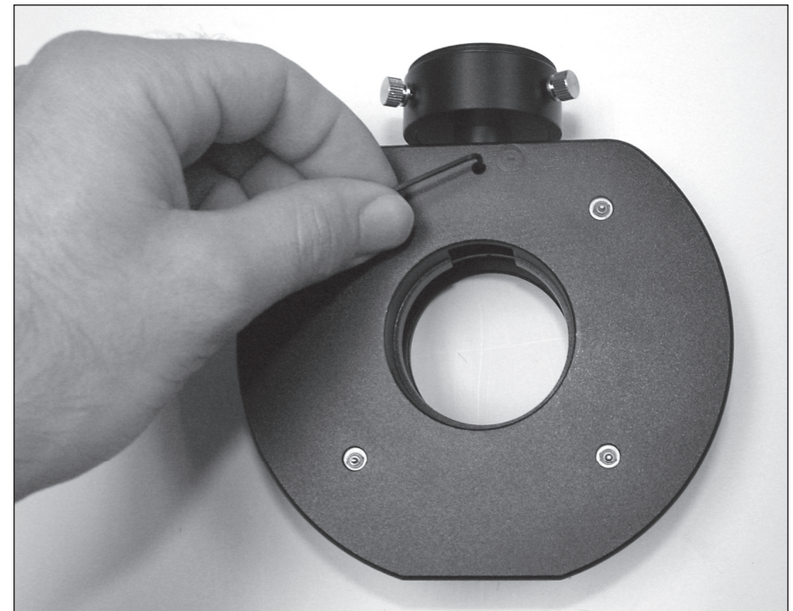
Figure 8. The prism can be lowered or raised in the "Z" axis by loosening the small hex screw in the back of the unit.
