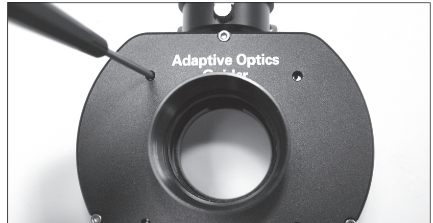
Figure 42. Use a flat head screwdriver to turn the jammed motor until it turns freely.
