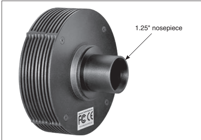
Figure 6. To use a CCD camera with the 8" f/4.0 Newtonian Astrograph, the camera must have a 1.25" or 2" nosepiece, which is inserted into the appropriate accessory holder in the focuser. An external camera adapter with T-threads could be used in lieu of the nosepiece.
