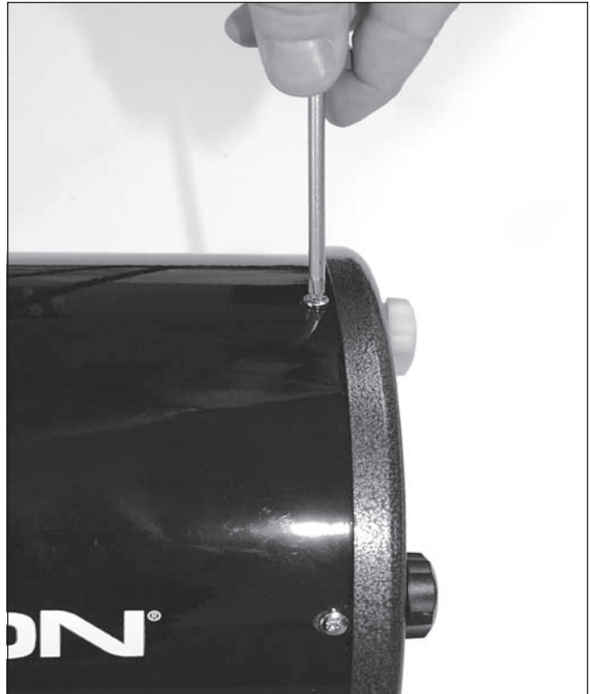
Figure 15. To clean the primary mirror, you must remove the mirror in its cell from the telescope tube. To do so, remove the six Phillips-head screws that fasten the rear cell to the tube. Then separate the cell from the tube.
