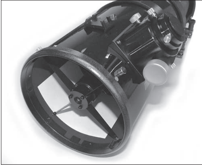
Figure 11. Placing a piece of white paper inside the optical tube opposite the focuser provides a bright background when viewing into the focuser.
