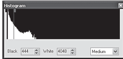
Figure 9. The sliders on the Histogram can be adjusted to reveal lighter or darker depths of the image.
