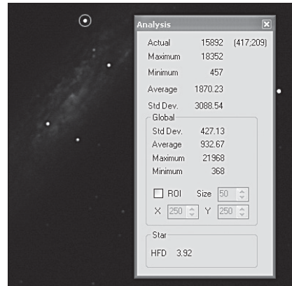
Figure 10. The Analysis window displays useful data about your image. Hovering the mouse over a star will also display the HFD value which indicates the star diameter for best focus.
