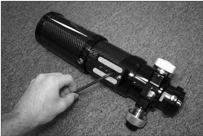
Figure 4.2. Using the included 5mm hex key, remove the 2 socket head screws to reverse the orientation of the mounting block to balance the telescope for heavier accessories.
