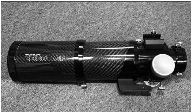
Figure 4.3. Orientation of the mounting block when reversed to balance the telescope for heavier accessories.
