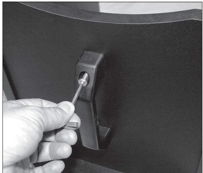
Figure 9. Use the Allen wrench and the two included machine screws to attach the handle to the front panel.
