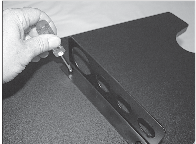
Figure 8. Install the eyepiece rack on the left side panel with the two small wood screws as shown.
