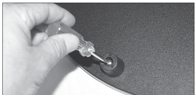
Figure 5. Install the three feet with the included screws on the bottom side of the bottom groundplate.
