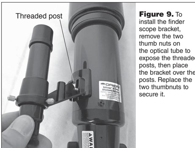
**Figure 9.** To install the finder scope bracket, remove the two thumb nuts on the optical tube to expose the threaded posts, then place the bracket over the posts. Replace the two thumbnuts to secure it.
