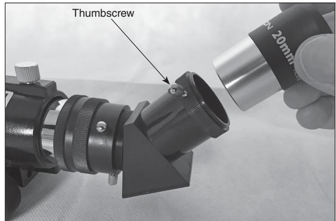
**Figure 11.** Insert the eyepiece into the diagonal and secure it with the thumbscrew.
