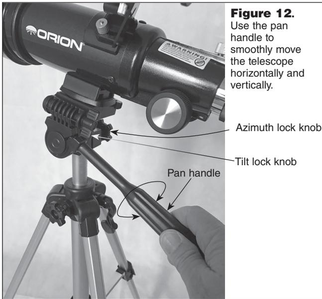
**Figure 12.** Use the pan handle to smoothly move the telescope horizontally and vertically.
