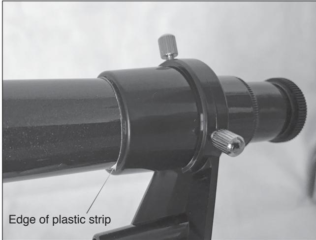
**Figure 8.** Slide the finder scope tube, eyepiece end first, into the bracket, making sure the plastic strip surrounds the tube. The strip should be just barely visible when the finder scope is fully inserted, as shown.
