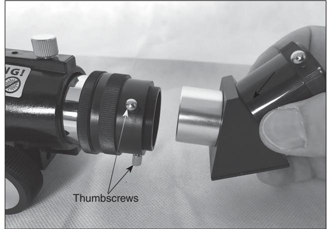
**Figure 10.** Insert the 45-degree correct-image diagonal into the focuser drawtube and secure it with the two thumbscrews.
