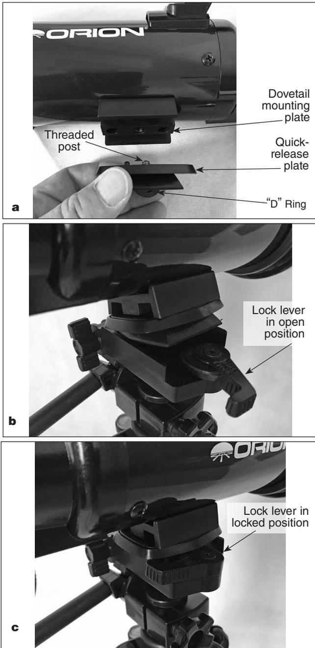
**Figure 6. a)** Attach the quick-release plate to the dovetail mounting plate on the telescope. **b)** Slide the quick-release plate into the pan head's saddle by tilting it and then pressing downward. **c)** Finally, close the lock lever to secure the telescope on the pan head.
