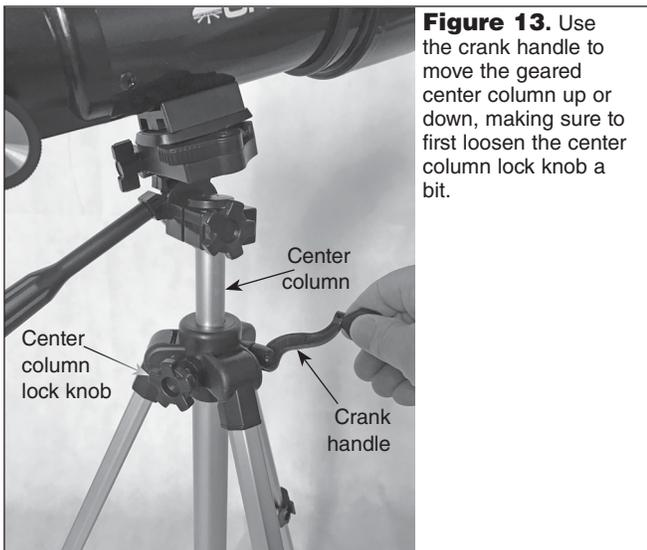
**Figure 13.** Use the crank handle to move the geared center column up or down, making sure to first loosen the center column lock knob a bit.
