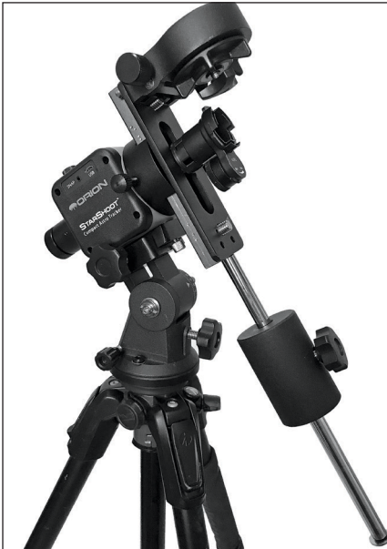
Figure 3. The combination of the Dec Bracket and optional Counterweight and Shaft allows proper counterbalancing of telescope or camera payloads.
