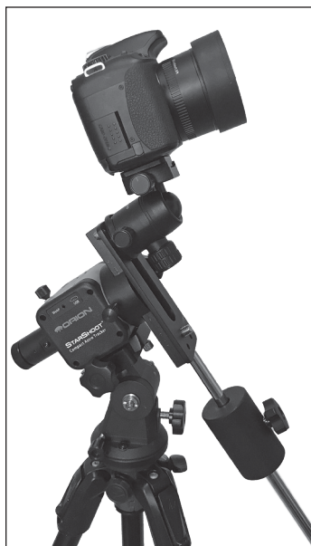
Figure 5. The declination platform can be removed and replaced with the Ball Head Mount.
