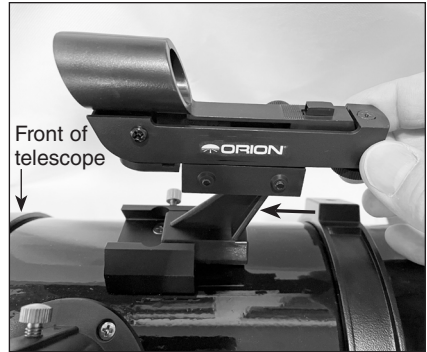
Figure 1. Slide the EZ Finder II into the telescope's finder scope base as shown.
