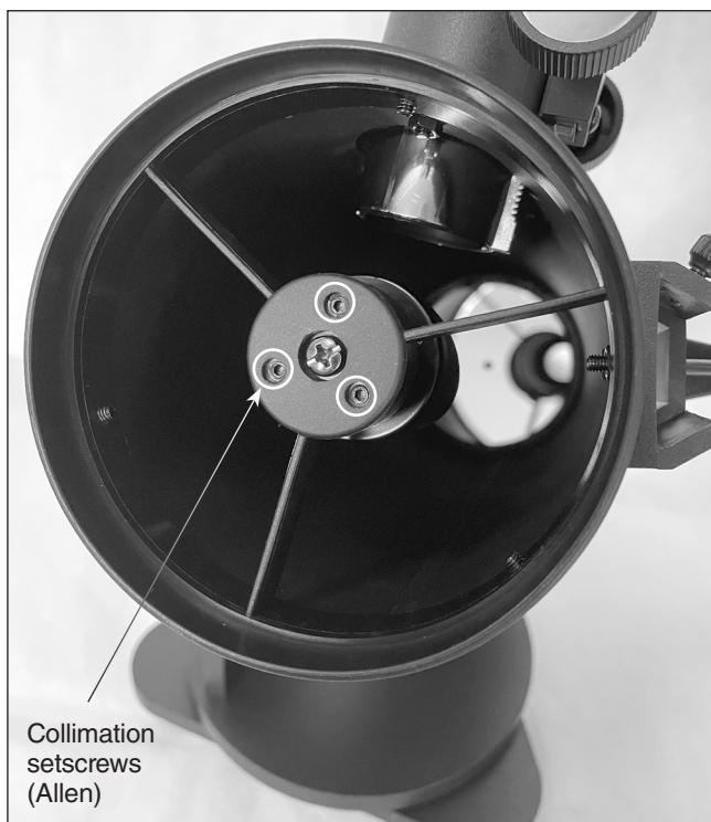
Figure 14. Use the included 2mm Allen wrench to adjust the three secondary mirror collimation setscrews.
