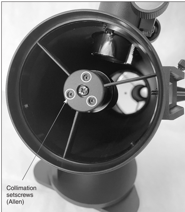
Figure 15. Use the included 2mm Allen wrench to adjust the three secondary mirror collimation setscrews.
