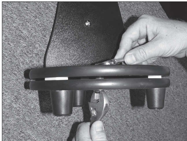
Figure 11. Making optional adjustments to the azimuth tension.
