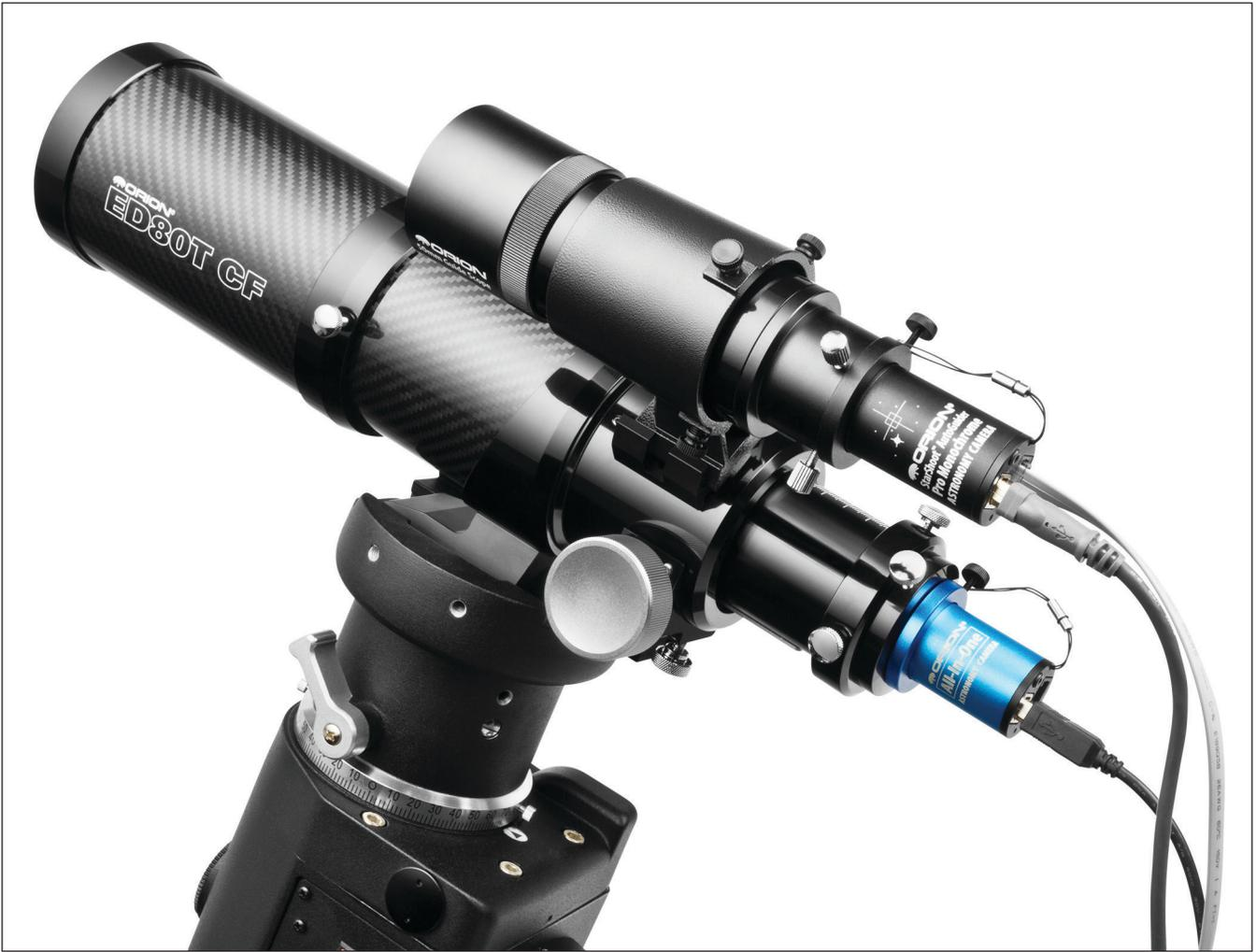
**Figure 15:** The All-In-One setup as the main imaging camera and the SAG PRO setup as an autoguider.
