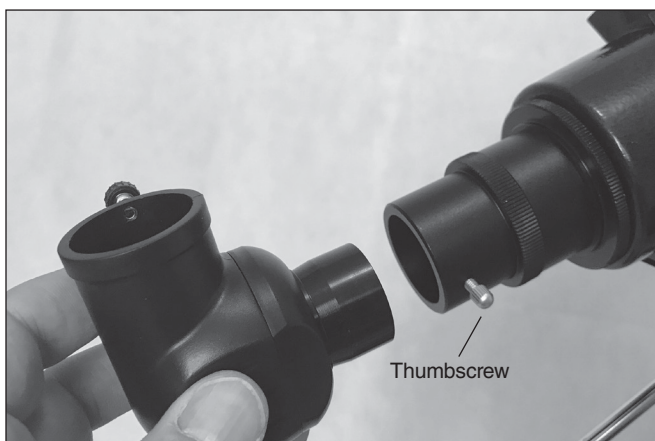
Figure 6. Insert the barrel of the correct-image 90-degree diagonal into the focuser drawtube and secure it with the thumbscrew.
