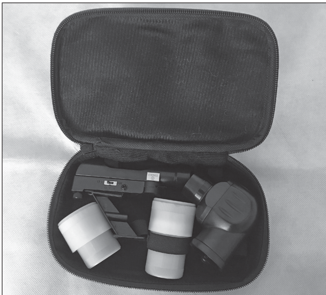
Figure 11. When not in use, store the two eyepieces in their bolt cases, the diagonal, and the red dot finder scope in the zippered accessory pouch.
