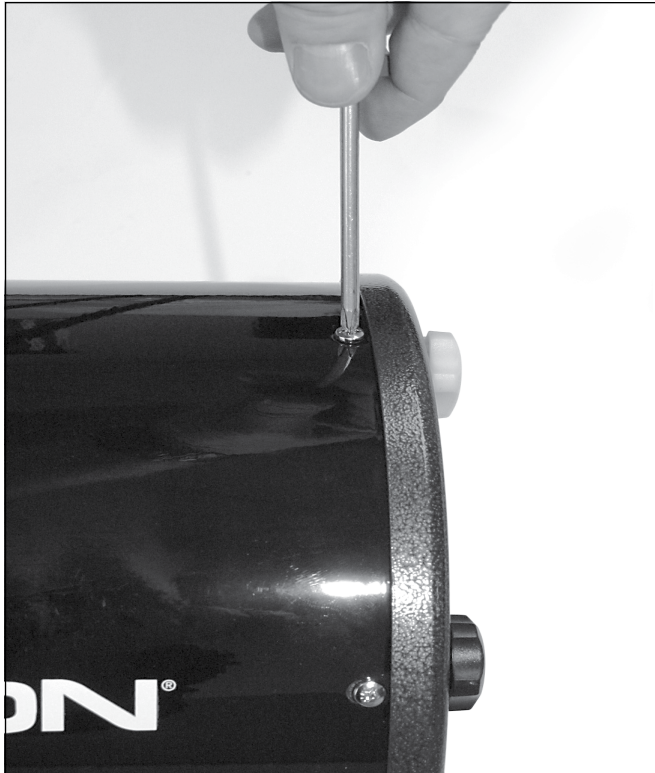
Figure 18. To clean the primary mirror, you must remove the mirror in its cell from the telescope tube. To do so, remove the six Phillips-head screws that fasten the rear cell to the tube. Then separate the cell from the tube.
