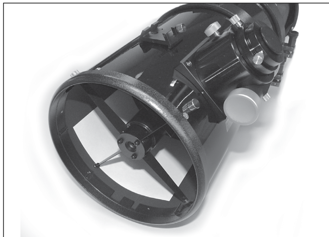
Figure 13. Placing a piece of white paper inside the optical tube opposite the focuser provides a bright background when viewing into the focuser.
