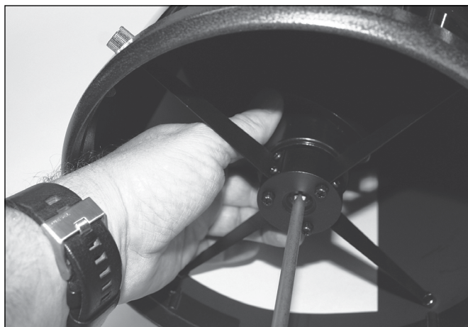
Figure 14. To center the secondary mirror axially under the focuser, hold the secondary mirror holder in place with your fingers while adjusting the center screw with a large Phillips-head screwdriver. Later you will adjust the tilt of the secondary mirror by turning the three small set screws that surround the large center screw.
