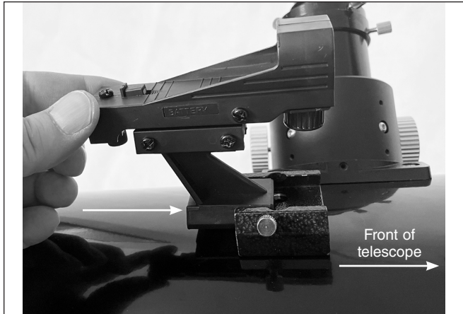
Figure 11. Slide the red dot scope's bracket into the dovetail base, then secure it with the thumbscrew.
