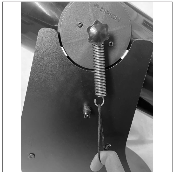
Figure 10. To attach the springs to the base, grip the pull loop and pull down on the spring until you can place the spring’s end ring over the screw head and onto the narrow part of the spring post. Then release the pull loop.
