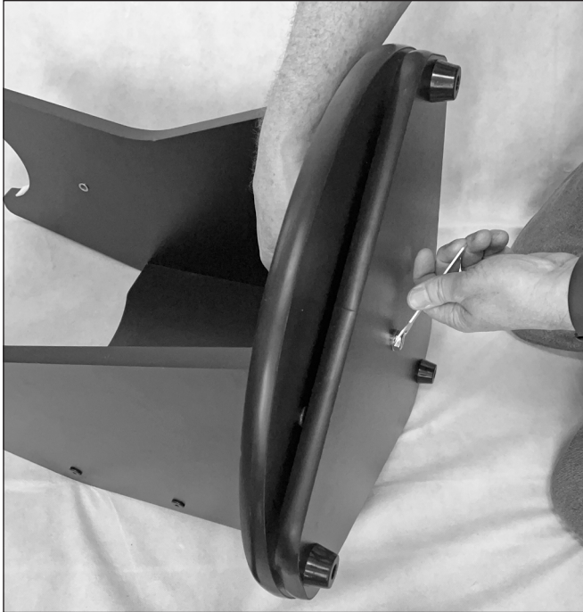
Figure 5. Once the bolt is inserted through the groundplate and top baseplate, place the second washer on the bolt and then thread on the lock nut. Use the two 17mm crescent wrenches to lightly tighten the nut..
